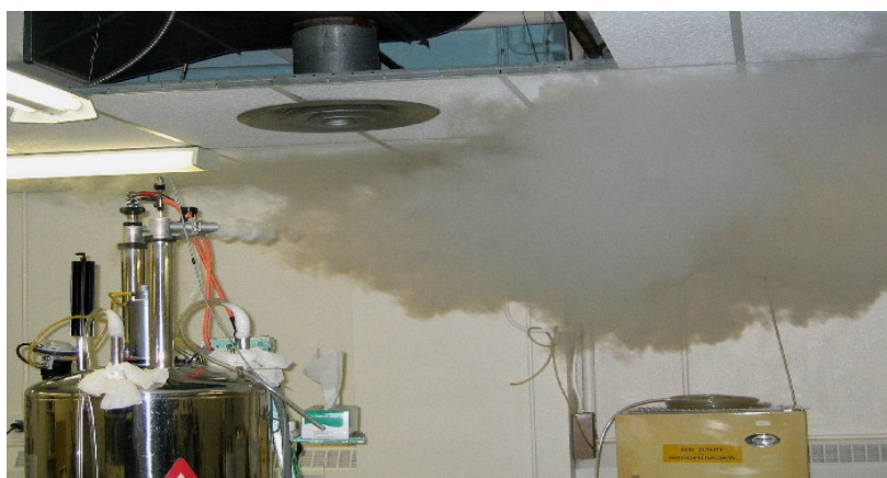
Figure 3 - April 10, 2003 a relatively small 200 MHz NMR magnet quench during decommissioning of the instrument.
