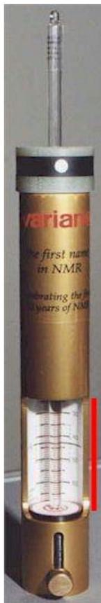
**Figure 4** Sample depth gauge. These are at all spectrometers. If a sample breaks contact staff for help, especially if it breaks in the depth gauge.
