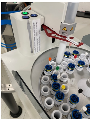
Figure 25 – The tube prevents access when a sample is in the magnet. Leave that spot alone.
