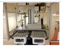
The new Agilent 7620 sample handing robot means that multiple over night and/or weekend experiments can be queued up without users having to be present. Notifications and status updates for users are handled identically to the other systems (*i.e.* m400 and u500 spectrometers) via email. Special thanks to Mark for setting up everything with a consistent user interface.
