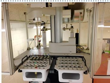
The new Agilent 7620 sample handling robot means that multiple overnight and/or weekend experiments can be queued up without users having to be present. Notifications and status updates for users are handled identically to the other systems (*i.e.* m400 and u500 spectrometers) via email. Special thanks to Mark for setting up everything with a consistent user interface.
